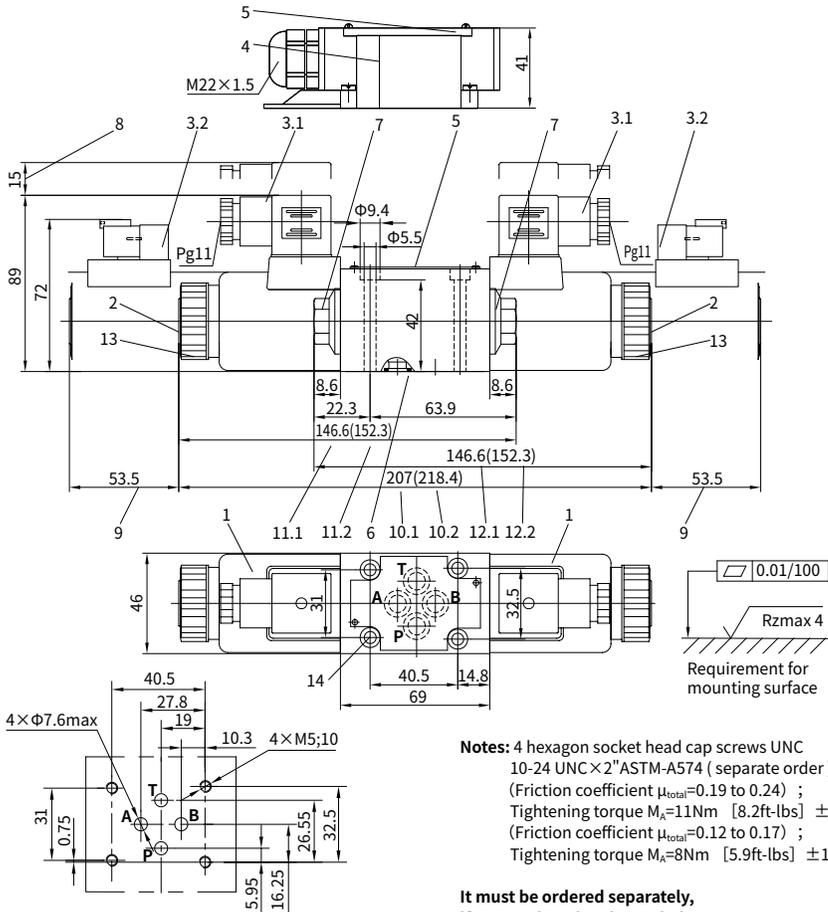
**Notes:** 4 hexagon socket head cap screws UNC 10-24 UNC  $\times$  2" ASTM-A574 (separate order)
